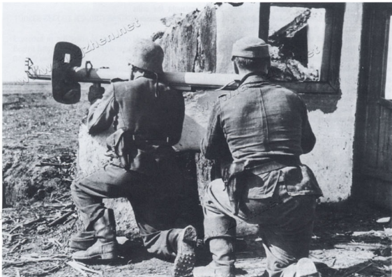
Above: The 88mm Panzerschreck close-combat anti-tank weapon was a copy of the American M1 bazooka, first seen in Tunisia. With a range of 150m, it was operated by a two-man team and proved very effective from its introduction in 1943.
